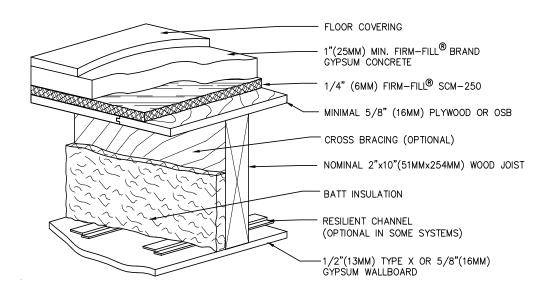
When installed over Nominal Wood Joist, 1" (25mm) FIRM-FILL<sup>®</sup> Brand Gypsum Concrete and 1/4" (6mm) FIRM-FILL<sup>®</sup> SCM-250 achieve excellent fire and sound ratings, while providing a superior crackresistant surface surface for the installation of finished floor coverings.
